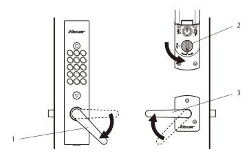
This diagram shows the righthanded configuration (it is symmetrical for left-handed configurations)
